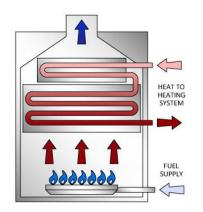
**Condensing** boilers work very similarly but rather than immediately exhausting the heated gas through the flue it is ran back over another section of coil to extract more heat. As the water absorbs this additional heat, the gas is further cooled. The cooling causes water to condense out of the air and into a drain pan and the gas is then exhausted through a flue. In the non-condensing, there is no condensation and therefore no drain pain is required.
