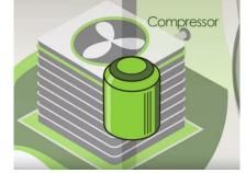
**Condenser Coil (Step 2):** At this point the high temp refrigerant leaves the compressor and enters into the condenser coil. As the refrigerant travels through the coil at a higher pressure, it becomes a liquid. This is called "changing state". Then outdoor air is pulled over the coil and the heat is absorbed into the outdoor air.
