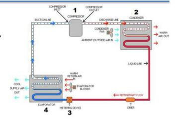
**Compressor (Step 1):** The compressor is the heart of the system. Just like your heart pumps blood through your body at a specific flow rate and pressure, the compressor pumps the refrigerant through the air conditioning system at a designed flow rate and pressure.
