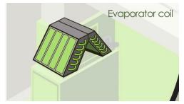
Now that the heat from the indoor air has been absorbed into the vapor refrigerant it must be transported back to the compressor and pumped into the condenser coil for the heat to be removed.
