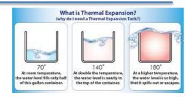
For example, water heated from 90°F to a thermostat setting of 140°F in a 40 gallon water heater will expand by almost one-half gallon. Since water is not compressible, the extra volume created by expansion must go somewhere.
